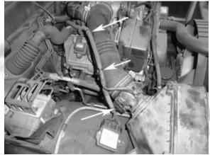
2- Remove the breather hose from the back of the stock intake. Loosen the clamp at the throttle body.
