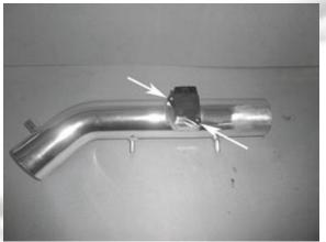
8- Install the rubber trim to the heat shield. Place the velocity stack adapter in the heat shield and install the supplied flex coupler with 2 clamps to the other side of it. Make sure the coupler is pushed completely against the heat shield. Once the adapter and coupler are tight against the heat shield,
