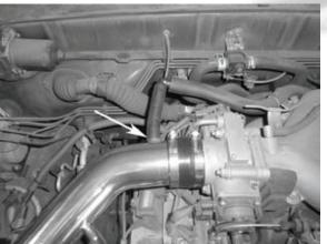
14- Reconnect the existing hose to the intake pipe. Using the supplied smaller hose, connect it between the engine and
