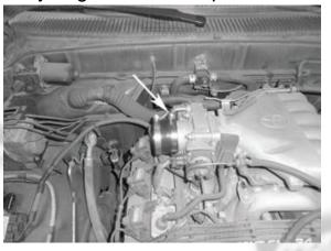
11- Install the intake pipe as shown and once it get in to the position, tighten the clamps on both side.
