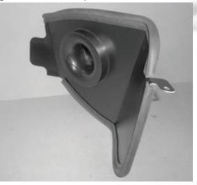
9- Install the eat shield into the vehicle. The arrow designated with "A" reuses the factory hardware. The 2 other locations use the supplied hardware.
