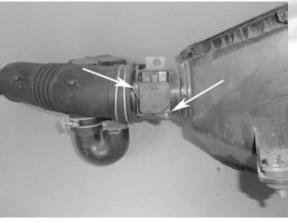
Insert and secure the MAF sensor onto the intake pipe with the provided screws.
