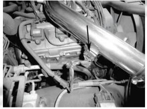
13- Using the bigger size hose and the 90 degree hose fitting, reconnect the vent line to the intake pipe.
