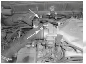
Disconnect the hose from the engine as shown in the picture and unclip the hose.
