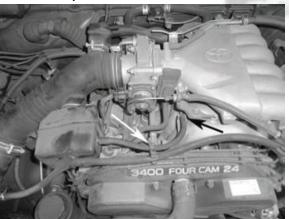
4- Disconnect the hose from the air box and unclip the hose.
