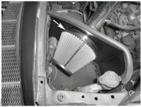
16-Make sure that all clamps and hardware are fully tightened. Start the vehicle and let it warm up. Shut off and inspect the installation once more for any loose clamps wires, or
