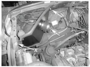
10- Install the supplied coupler with 2 clamps on the throttle body. Tighten the clamp on the throttle body at this point.
