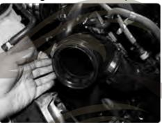
17- Install the provided coupler with 2 clamps to the secondary turbo housing. Tighten the clamp on turbo housing side.
