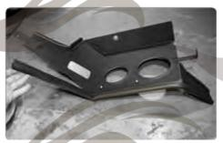
12- Locate the stock air box grommet and install the provided stand-off stud to the grommet. Make sure to secure it.
