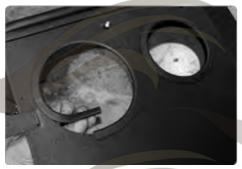
11- Install the thick rubber trim to heatshield. Note: Longer trim, notch for better corner installation.
