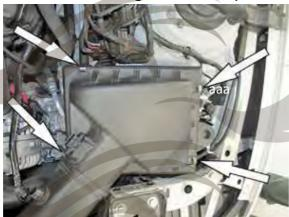
6- Lift up and remove the lower air filter box housing from the inner fender.
