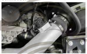
16- Install the provided air filter and secure with the clamp on the filter neck.
