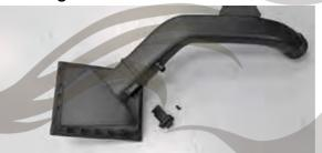
13- Install the mass air flow sensor into the provided intake pipe and secure with the provided hardware.
