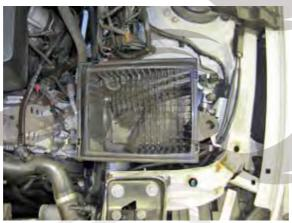
7- Install the filter adapter into the heat shield and secure with the provided bolts.
