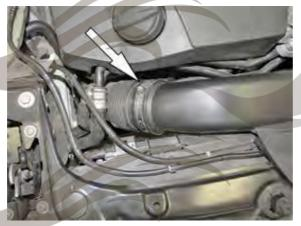
5- Release the 4 clips that securing upper air filter box housing to the lower housing. Lift off and remove the intake tube/air filter box housing and stock panel air filter.
