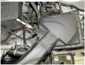
3- Disconnect the crank case vent line from the port on the stock intake tube.
