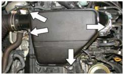
4. Unlatch the upper air box retaining clips, disconnect the fuel pressure regulator and then lift the intake tract off of the throttle
