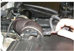
2. Remove the 2 bolts that secure the pressure sensor to the stock intake tube. **NOTE: These bolts will be reused in a later step.**
