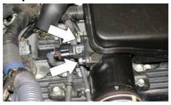
3. Remove the 3 bolts that secure the intake plenum to engine and loosen the throttle body hose clamp.
