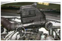
6. Remove the three lower air box retaining blots shown and then remove the lower air box from the vehicle. **NOTE: We recommends that customers do not discard the stock air intake.**
