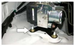
11. install the heat shield onto the vehicle and secure with the provided hardware and the nut remove in step #10.
