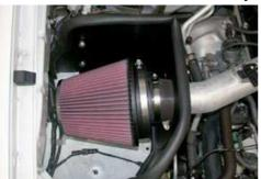
24. Clip the mass air flow sensor wire harness retainer into the pipe mounting bracket.
