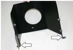
8. Install the small heat shield mounting bracket with the provided spacer onto the heat as shown.
