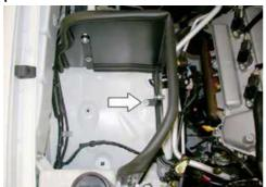
12. remove the 2 valve cover bolts shown. **NOTE: These bolts will be reused.**
