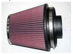
22. Install the provided reducer coupler onto the filter assembly and secure with the provided clamps.
