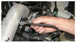
20. Install the provided hose(large) onto the valve cover port and then onto the intake pipe.
