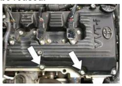
13. install the tube mounting bracket assembly onto the valve cover using the factory bolts removed in step #12.
