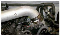
18. Secure the intake pipe to the pipe mounting bracket with the provided hardware and then tighten the hose clamp at the throttle body.
