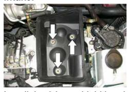
7. Install the 2 heat shield brackets onto the heat shield as shown with the provided hardware.
