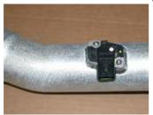
17. Install the intake pipe onto the throttle body and align with the mounting bracket that was installed in step #13.
