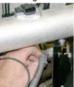
25. Reconnect the mass air flow sensor electrical harness.
