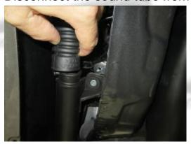
19- Remove the resonator from the vehicle.
