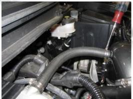
41- Make sure there is proper clearance around the intake system and then tighten the bolt on the middle intake pipe
