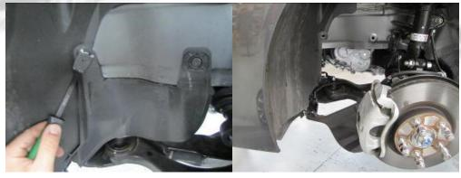
13- Remove the philips screw on the weather guard.
