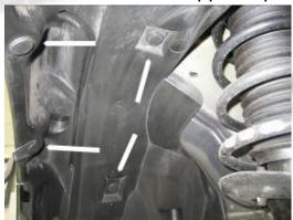
15- Remove the 2 bottom clips that hold the splash shield.
