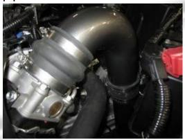
33- Remove the OEM bolt that holds the ground wires and replace it with a rubber spacer.
