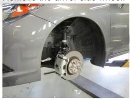
12- Remove the 2 plastic clips securing the side splash shield, and then move the shield out of the way.
