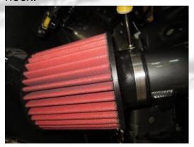
38- Make sure the filter has proper clearance and then tighten the clamps on the lower intake pipe.
