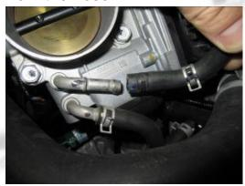
24- Relase the clip on the thermostat collant hose and pull the hose off. The stock clips will be reused. NOTE: Please make sure your vehicle is cold because coolant will spill out from the hose.
