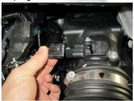
2- Release the MAF sensor clip from the air box.
