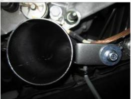
32- Install the upper pipe onto the throttle body and the middle pipe.
