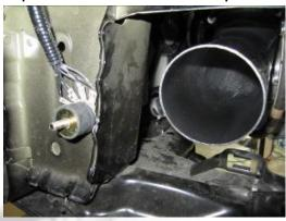
34- Install the provided reducer coupler with 2 clamps onto the lower intake pipe. Semi-tighten both clamps.
