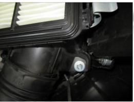
8- Lift up on the back of the lower air box and then remove it.
