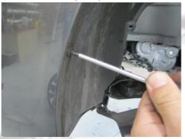
14- Remove the 4 front upper clips that secure the splash shield.
