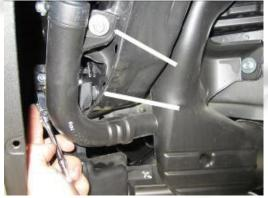
18- Disconnect the sound tube from the resonator.
