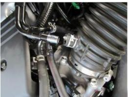
4- Loosen hose clamp on the throttle body.
