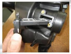
28- Install the MAF sensor to the upper intake pipe.
