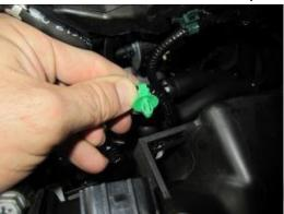
3- Release the clip on the PCV pipe and remove the pipe from the intake tube. Remove the PCv pipe from the valve cover.
