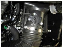
6- Remove the stock intake tube and the air box lid.
