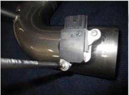
29- Install a provided reducer coupler with 2 clamps on the upper intake pipe and tighten the clamp on the pipe and
