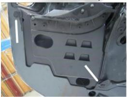
16- Move the splash shield out of the way.
