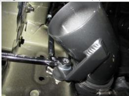
37- Install the provided air filter. Tighten the clamp on the filter neck.
