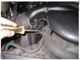
4- Loosen the hose clamp securing the intake duct to the MAF sensor.
