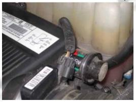
3- Disconnect the plastic mount securing the radiator hose to the intake duct.
