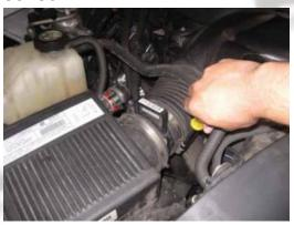
5- Remove the bolt securing the engine cover.
