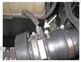
27- Install the air filter on the air horn.
