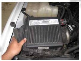
12- Remove the 5 bolts securing the metal air box tray. Put the bolts aside, some of them will be reused again.
