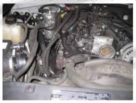
11- Pull up on the stock air box to disengage it from the plate on the bottom.
