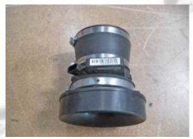
26- Install the MAF sensor assembly created in the previous steps onto the intake pipe, and then re-connect the MAF sensor harness to the MAF sensor.
