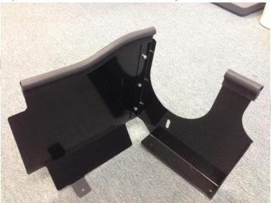
17- Install the heat shield over the air box tray was and line up the holes.
