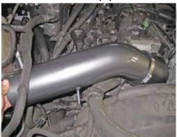
22- Align the bracket with the rubber mount installed in step 17.
