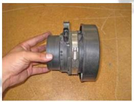
25- Install the coupler on the MAF sensor and secure with the supplied clamp and loosely install the last clamp on the other end.
