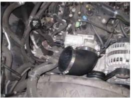
21- Install the intake pipe into the coupler.
