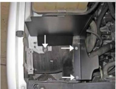
19- Install the rubber spacer using the supplied big washer and big nut on the heat shield.
