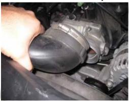
9- Disconnect the intake duct from the MAF sensor.
