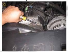
8- Pull the intake duct away from the throttle body.
