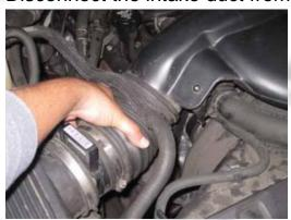
10- Remove the intake duct from the vehicle.
