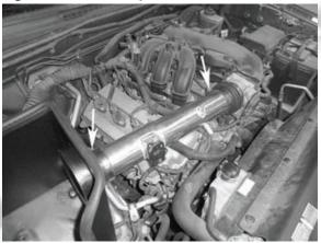
13. Connect the MAF sensor connector and the vent hose.
