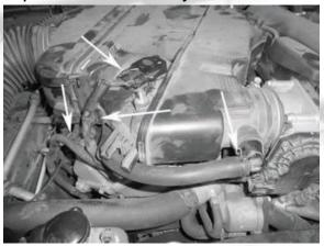
3. Remove the MAF sensor from the factory air box.
