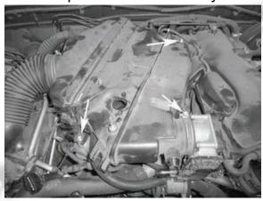
5. Remove the 2 screws securing the resonator.
