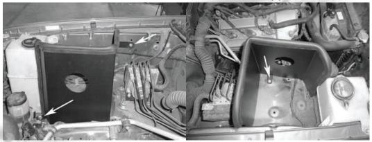
11. Install the flex coupler with 2 clamps on the throttle body. Tighten the clamp on the throttle body at this point.
