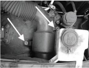
6. Move the air box so it comes off the throttle body. Remove the vacuum hose on the fuel regulator. Lift and remove the entire
