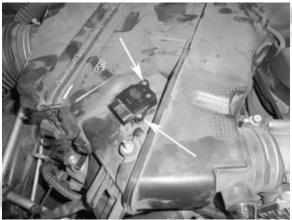
4. Remove the 2 mounting screws on the stock air box and loosen the clamp at the throttle body.
