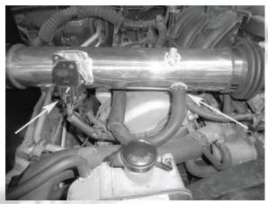
14. Install the supplied vaccum hose from the vacuum port on the pipe to the fuel regulator.
