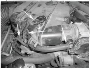
3. Remove the MAF sensor from the factory air box.
