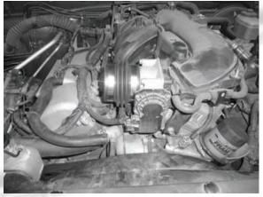
12. Install the open end of the intake pipe into the flex coupler on the throttle body. Install the velocity adapter in the heat shield and once in place, slide the coupler from the long side of the intake onto the velocity adapter. Once the pipe in place,
