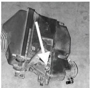
17. Install the factory engine cover. Rotate the intake tube to align the stud with the hole in the cover. Remove the engine cover and fully tighten the clamp at the throttle body. There is a small tab attached to the bottom of the cover that may need to
