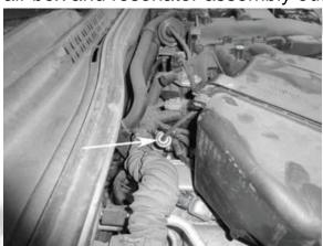
7. Loosen the 10mm nut that is on the clamp for the rubber mount. Then remove the 10mm bolt that secures the A/C line bracket. Remove the 12mm bolt in the power steering reservoir bracket. Rotate the A/C line bracket and line up the hole with the power steering reservoir bracket. Reinstall the bolt through both brackets and tighten. Tighten the nut on the clamp.
