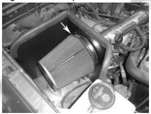
16. Use a Torx 6 or 4mm socket to remove the stud in the stock air box and install it in the threaded boss on the intake pipe. This stud will be used to reinstall the factory engine cover. Install this threaded stud into the threaded bung of the intake pipe.
