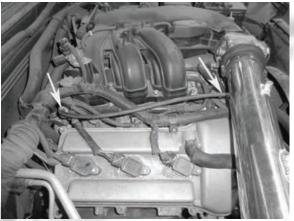
15. Install the air filter to the open end of the velocity adapter. Tighten the clamp on the filter neck.
