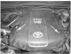
18. Reinstall the engine cover. Make sure that all clamps and hardware are fully tightened. Reconnect the battery cable, start the vehicle and let it warm up. Shit off and inspect the installation one more time for any loose clamps, wires, or hardware.
